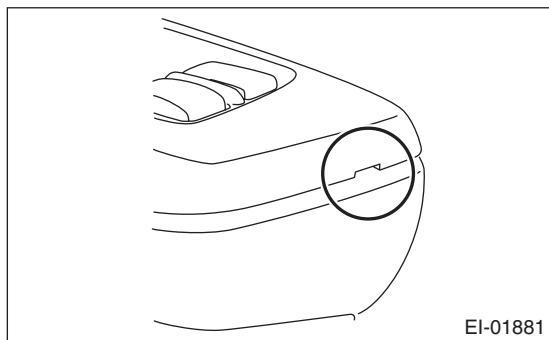
(3) Remove the side claws by using a plastic remover.
