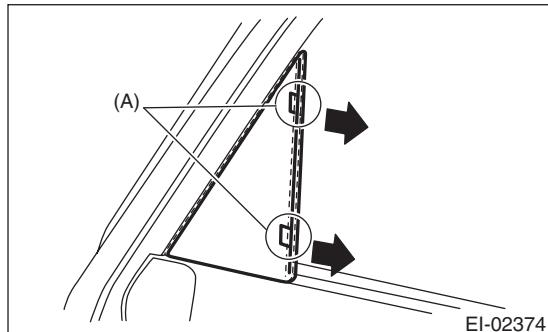
(2) Insert a plastic remover into the position shown in the figure while retaining the condition in step (1), and lift up the gusset cover.
