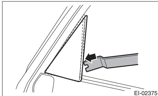
(3) Remove the gusset cover in the direction of the arrow to detach the clip section.
