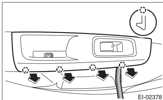
(4) Disconnect the harness connector, and remove the power window switch panel.
