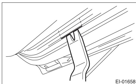
(2) Attach the protective tape (a) to the front door sash.
