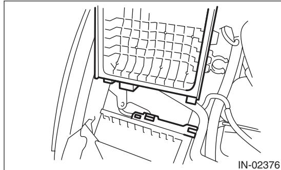
2) Remove the air intake duct. <Ref. to IN(H4DOTC)-11, REMOVAL, Air Intake Duct.>
