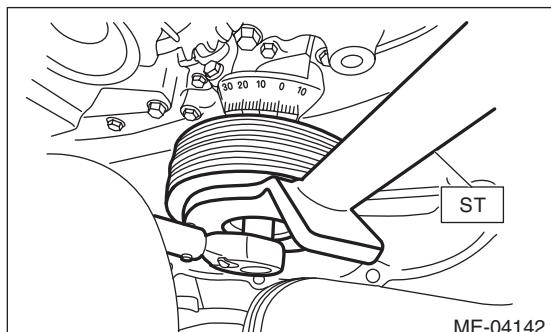
(2) Draw reference lines (A) and (B) using a marker to set the socket to the crank pulley bolt as shown in the figure.
