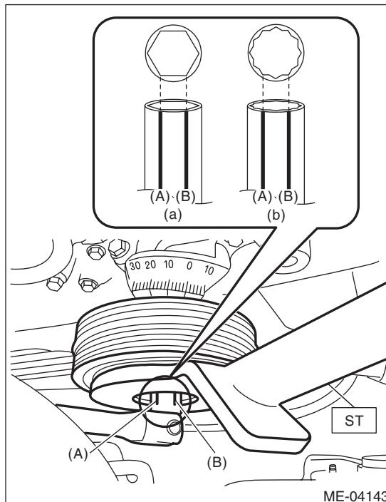
(a) When using 6-point socket
