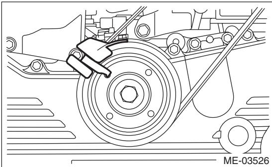
15) Remove the belt stopper from the compressor bracket.
