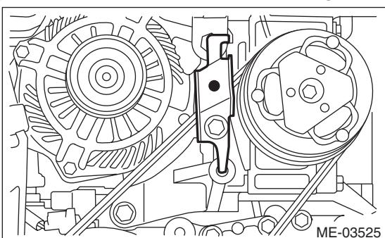
16) Make sure that the belt rib is securely installed on the groove of each pulley, then turn the crank pulley slowly, twice in the clockwise direction, to seat the rear side belt properly.
