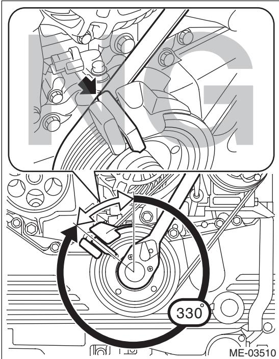
14) Remove the belt guide and belt guide holder from the crank pulley.
