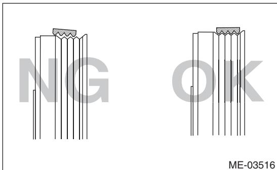
(3) The rib of the rear side belt is securely placed on the groove of the crank pulley.
