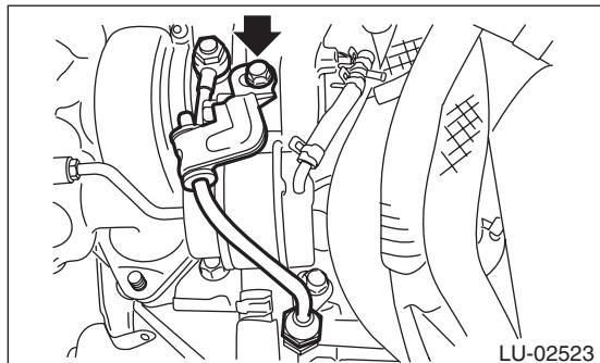
9) Connect the air control hose (A), and install the turbocharger to the intake duct.
