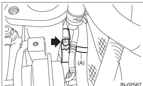
10) Connect the engine coolant hoses to the coolant filler tank.
