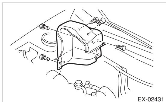
2) Remove the turbocharger upper cover.
