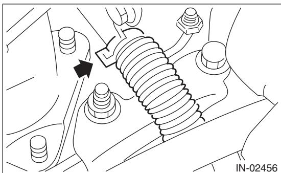
4) Temporarily tighten the bolts which secure the oil inlet pipe to the turbocharger. (except for WRX-SS model)
