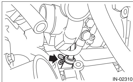
3) Connect the engine coolant hoses to the water pipe.
