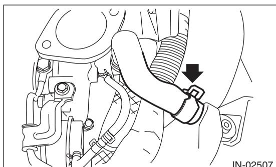
11) Install the joint pipe to turbocharger.
