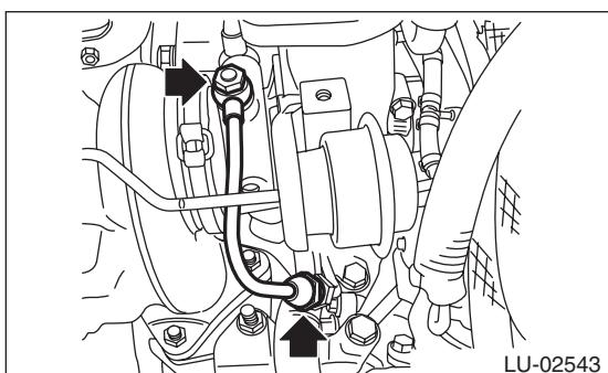
6) Tighten the bolts which secure the oil inlet pipe to the turbocharger. (except for WRX-SS model)
