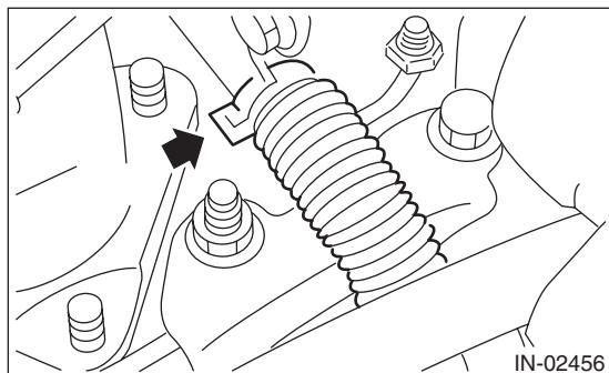
14) Disconnect the oil outlet hose from the oil outlet pipe, and remove the turbocharger.
