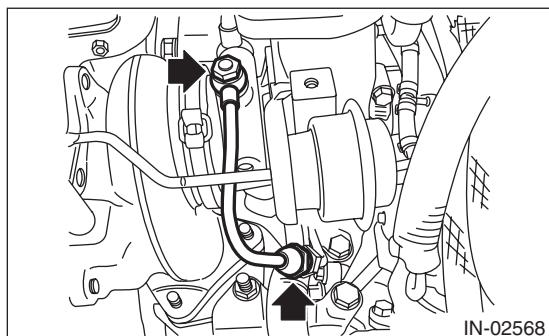
13) Disconnect the engine coolant hose from the water pipe.
