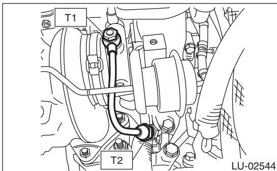
8) Tighten the bolts which hold the oil inlet pipe stay to the turbocharger. (except for WRX-SS model)
