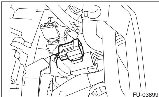
19) Connect the vacuum hose (A) and the connector (B) to the PCV hose assembly.
