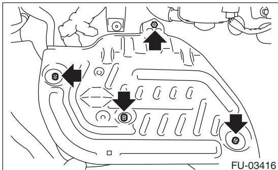
5) Remove the nuts and bolts which hold the ECM to the bracket.
