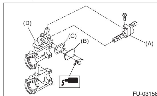
(A) Oil flow control solenoid valve
