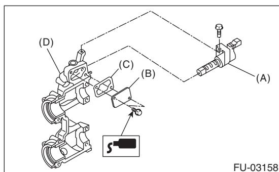
(A) Oil flow control solenoid valve
