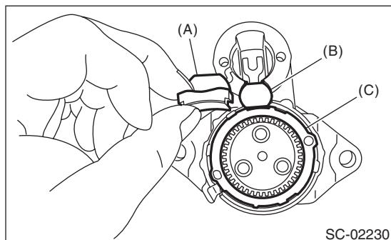
7) Assemble the armature assembly to the yoke assembly.
