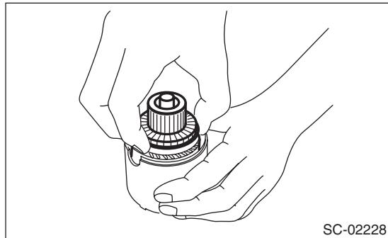
8) Attach the armature assembly and yoke assembly to the starter housing assembly together as a single unit.
