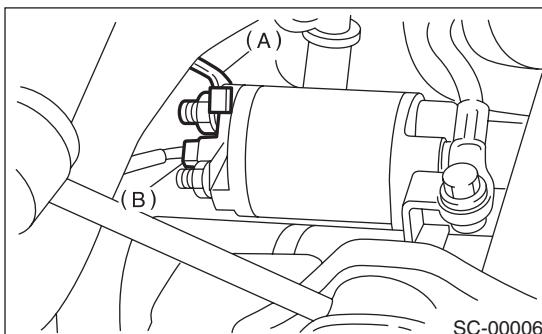
6) Remove the starter from transmission.
