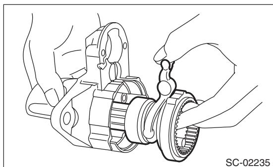
10) Use the following procedures to remove the overrunning clutch from the shaft.
