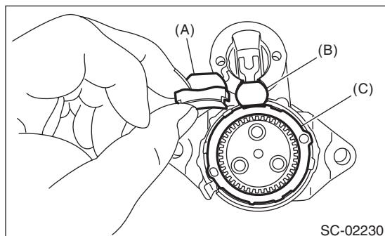
9) Lightly tap the starter housing assembly with a plastic hammer as shown in the figure, and remove the overrunning clutch, internal gear assembly, shaft and shift lever together as one unit.
