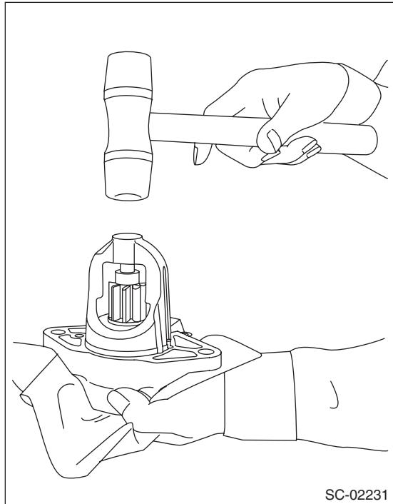
(1) Use an appropriate tool (such as a fit socket wrench), and remove the stopper from snap ring by lightly tapping the stopper with a plastic hammer.
