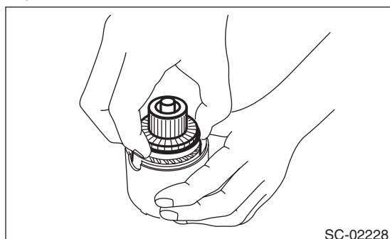
7) Remove the pinion gear from the internal gear assembly.
