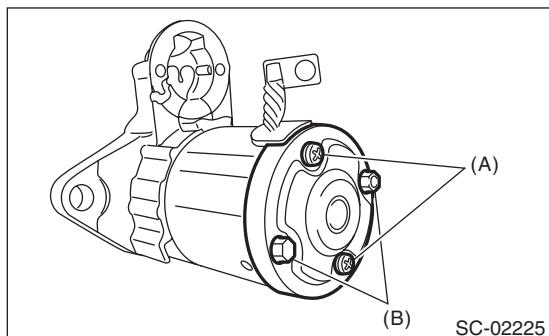
4) Remove the brush holder assembly from the armature assembly.
