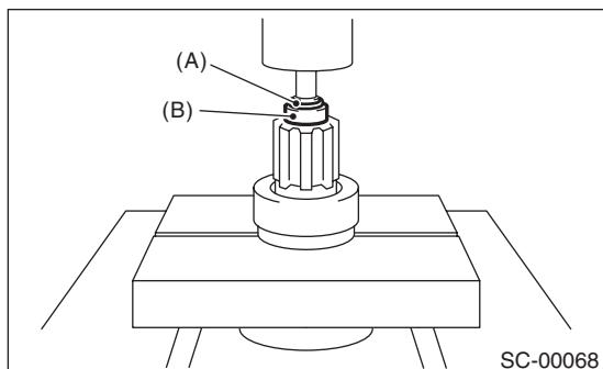
4) Assemble the overrunning clutch, internal gear assembly, shaft and shift lever as a single unit into the starter housing assembly.
