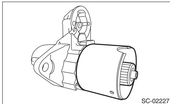
6) Separate the armature assembly and yoke assembly.
