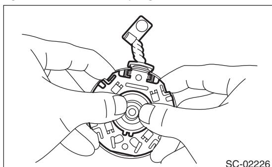
5) Remove the armature assembly and yoke assembly from the starter housing assembly together as a single unit.
