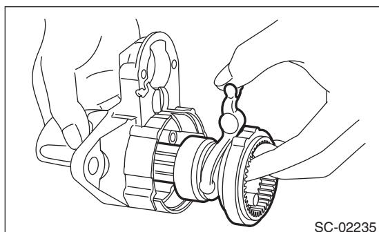
5) Apply grease to the inside of the internal gear assembly and pinion gear, and attach the pinion gear to the internal gear assembly.
