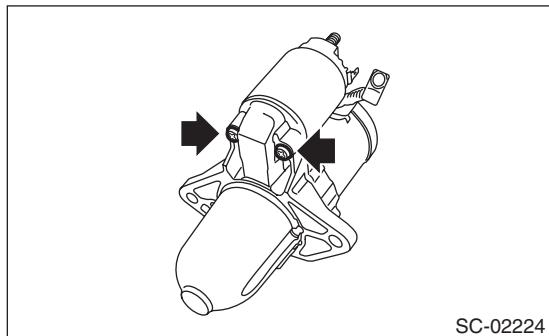
3) Remove screws (A) of the brush holder assembly, and through bolts (B) on both sides, and remove the starter cover assembly.
