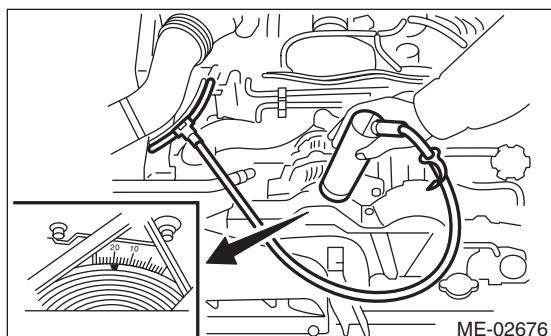
If the timing is not correct, check the ignition control system. <Ref. to EN(H4SO)(diag)-2, Basic Diagnostic Procedure.>
