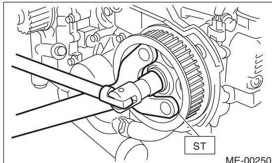
ST 499207400 CAM SPROCKET WRENCH
