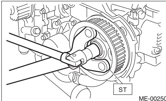
ST 499207400 CAM SPROCKET WRENCH
