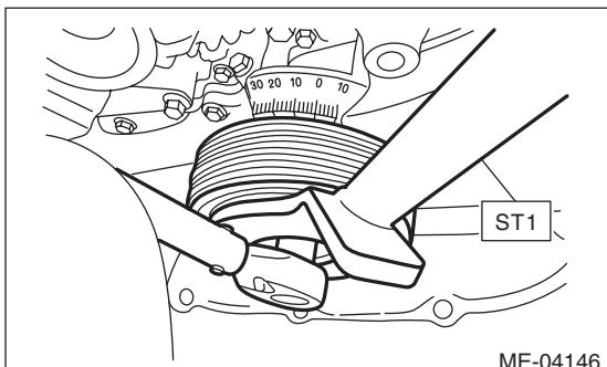
(3) Set the ST2, use the ST1 to lock the crank pulley, and tighten the crank pulley bolt to the specified angle.
