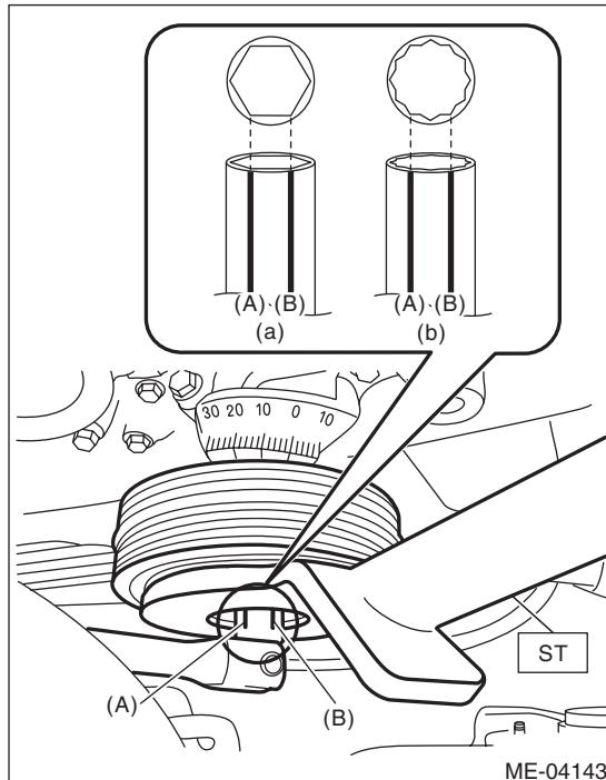
(a) When using 6-point socket
