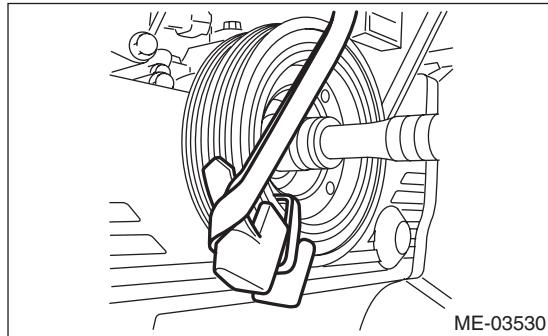
13) Slowly turn the crank pulley clockwise, and install the rear side belt.
