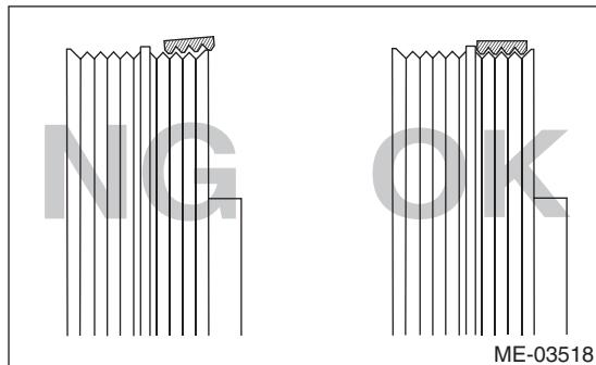
(4) The surface of the rear side belt is held by the belt stopper.
