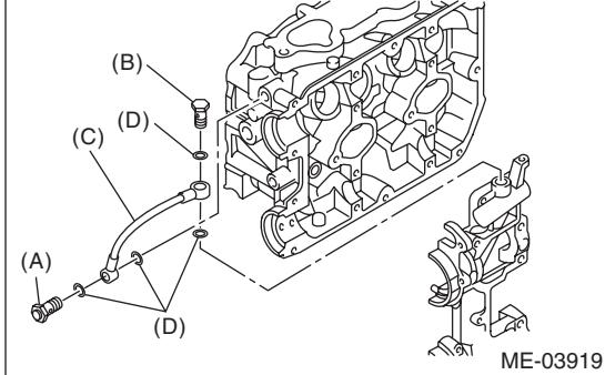
(A) Union screw with filter (with protrusion)
