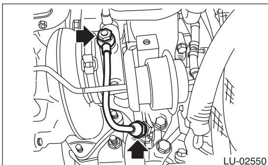
13) Tighten the oil inlet pipe of the turbocharger.
