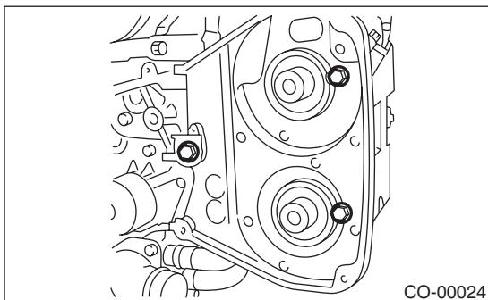
4) Install the cam sprocket LH. <Ref. to ME(H4DOTC)-59, INSTALLATION, Cam Sprocket.>
