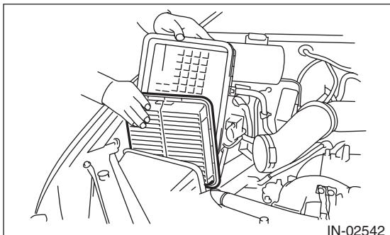
7) Remove the bolt (A) and nut (B) which secure the air cleaner case (front) to the body.
