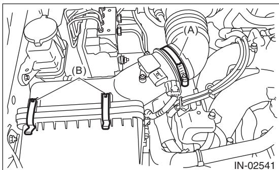
6) Remove the air cleaner case (rear) and air cleaner element.
