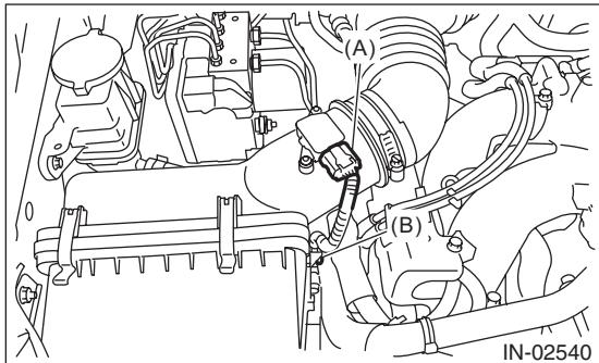
4) Loosen the clamp (A) which connects the air cleaner case to intake boot.
