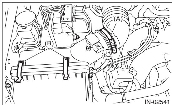
4) Connect the connector (A) to the mass air flow and intake air temperature sensor, and fasten the harness to clip (B).
