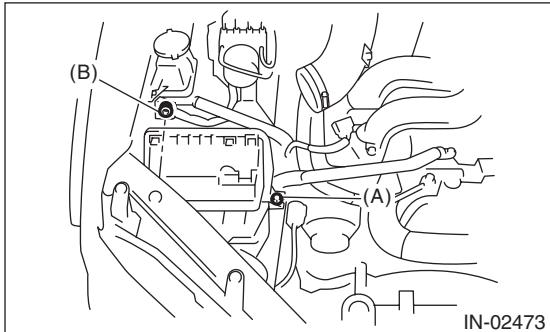
2) Install the air cleaner case (rear) and air cleaner element.
