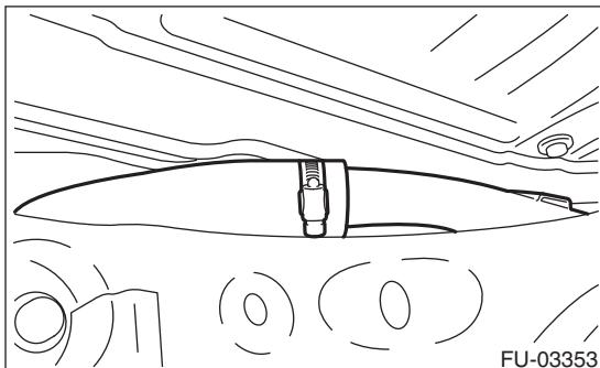
7) Set the container under the vehicle and insert the gasoline proof hose ( $\phi 10$  or less) into the fuel filler hose to drain the fuel.
