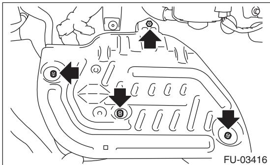
5) Remove the bolts and nuts which hold the ECM to the bracket.
