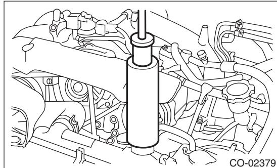
2) Apply a pressure of 157 kPa (1.6 kg/cm<sup>2</sup>, 23 psi) to the radiator and check the following points:
