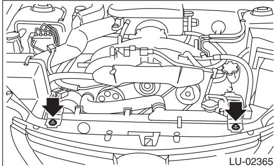
16) Lift the radiator up and remove the radiator from vehicle.
