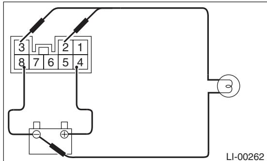
Replace the turn signal & hazard module if faulty.
