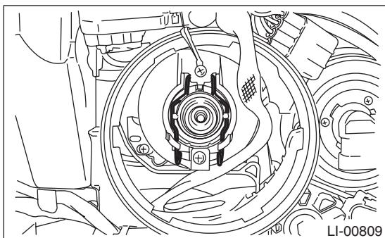
(3) Install bulbs with the same number of operating hours on both headlights, and light for approximately 30 minutes. Check for whether there is a difference in brightness on the right and left sides.
