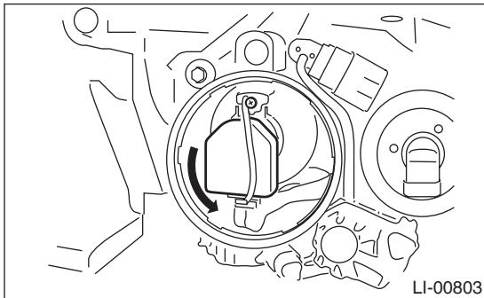
5) Remove the light bulb retaining spring, and remove the bulb.
