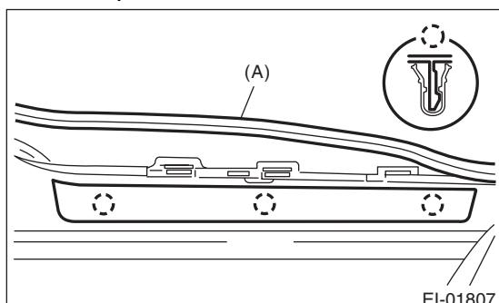
3) Remove clip (A), and remove the front pillar lower trim.
