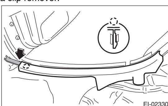
6) Remove weather strip (A) and door catcher cover (B), then remove the outside scuff plate.
