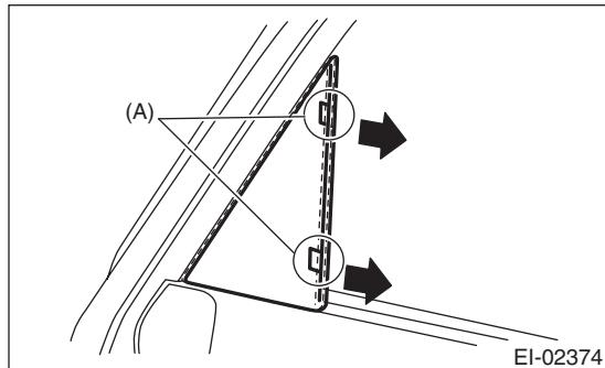
(2) Insert a plastic remover into to the position shown in the figure while retaining the condition in step (1), and lift up the gusset cover.
