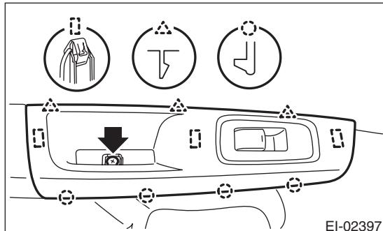
(1) Open the cover and remove the screws.
