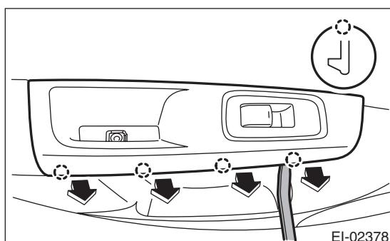
(4) Remove the power window switch panel.
