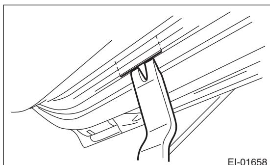
(2) Remove the cable (1) and (2) from the cable holder of inner remote.
