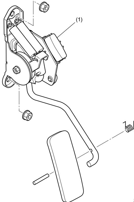
(1) Accelerator pedal position sensor
