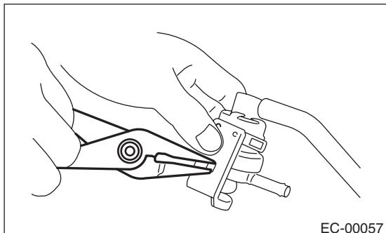
9) Disconnect the vacuum hose from pressure control solenoid valve.
