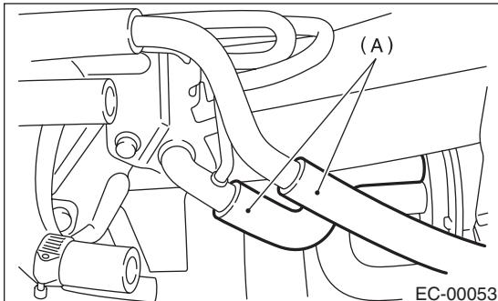
4) Remove the bolt which installs pressure control solenoid valve holding bracket on body.
