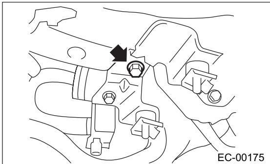
7) Remove the drain valve from bracket.
