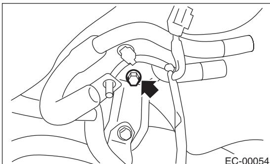
5) Disconnect the connector from pressure control solenoid valve.
