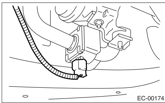
5) Disconnector the evaporation hoses (A) from joint pipes.
