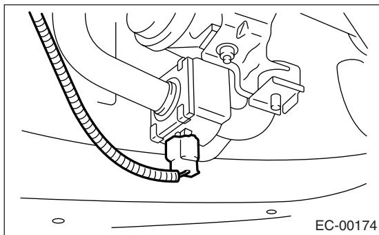
5) Disconnect the evaporation hoses from drain valve.
