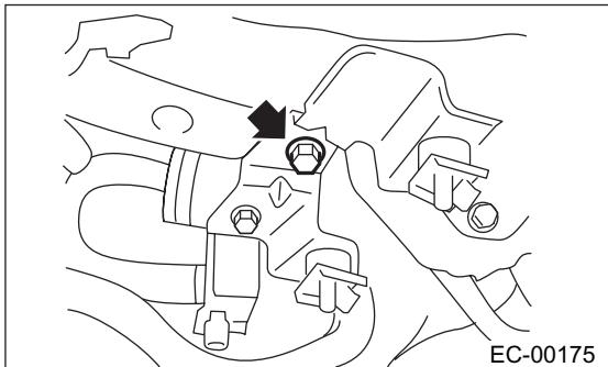
7) Disconnect the evaporation hoses, and remove the drain filter from the bracket.
