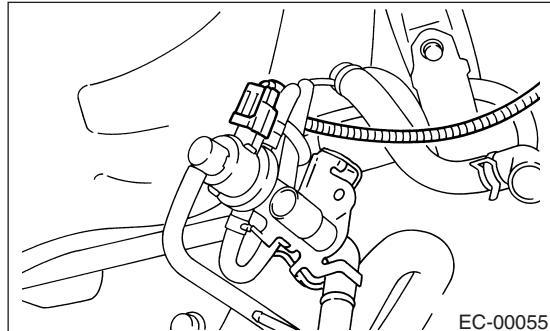
6) Disconnect the two evaporation hoses from pressure control solenoid valve.
