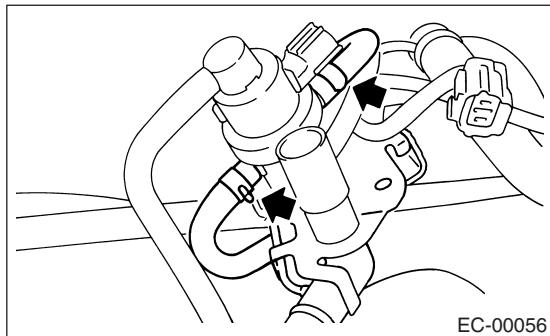
8) Remove the pressure control solenoid valve from bracket.
