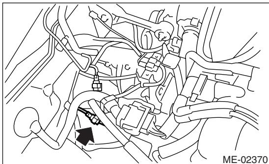
3) Disconnect the rear oxygen sensor connector.
