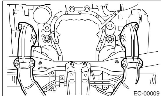
8) Remove the bolt which installs the front and center exhaust pipe assembly to hanger bracket.
