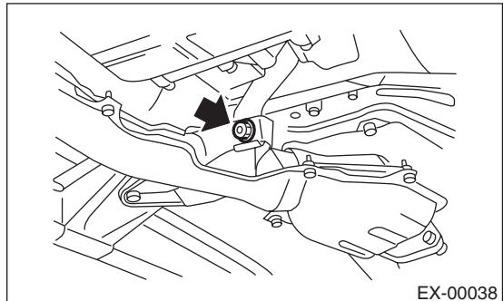
9) Remove the front and center exhaust pipe assembly from vehicle.
