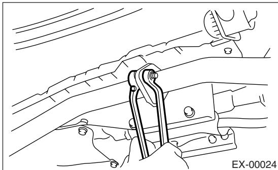
2) Apply a coat of spray type lubricant to the mating area of cushion rubbers in advance.
