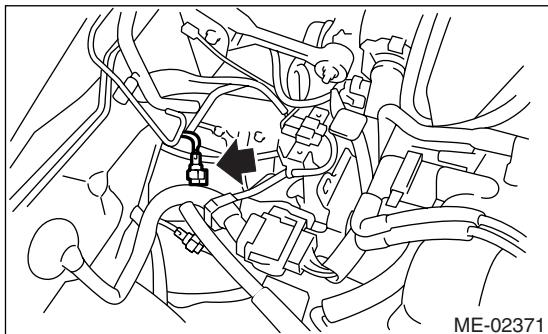
11) Connect the front oxygen (A/F) sensor connector.
