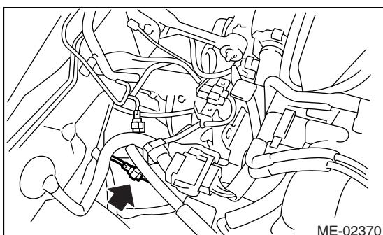
12) Connect the ground cable to battery.
