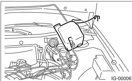
5) Disconnect the connector from ignition coil.
