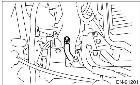
10) Use the TCM mounting stud bolts at the grounding point, when measuring voltage and resistance inside the passenger compartment.
