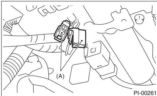
5) Connect the Subaru Select Monitor to data link connector located in the lower portion of instrument panel (on the driver's side).
