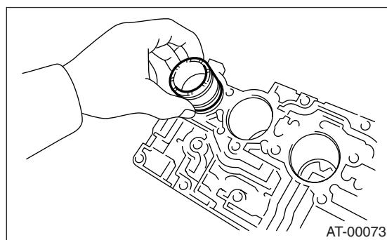
4) Install the spring and four steel balls to specified positions of upper valve body.
