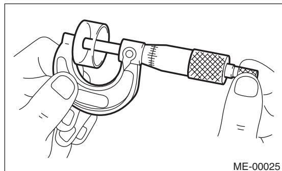
5) Based on the measured valve clearance and valve lifter thickness, obtain the correct amount of shims from the following table.
