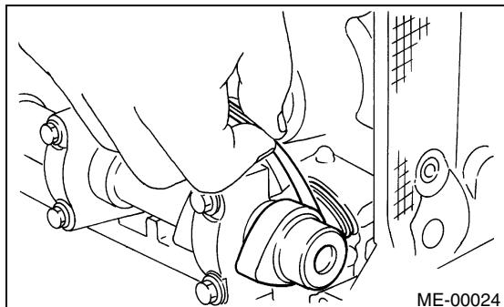
2) Remove the camshaft.<Ref. to ME(H4DOTC)-59, REMOVAL, Camshaft.>
