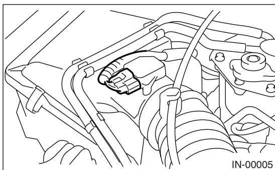
3) Loosen the clamp (A) which connects air intake boot to intake duct.
