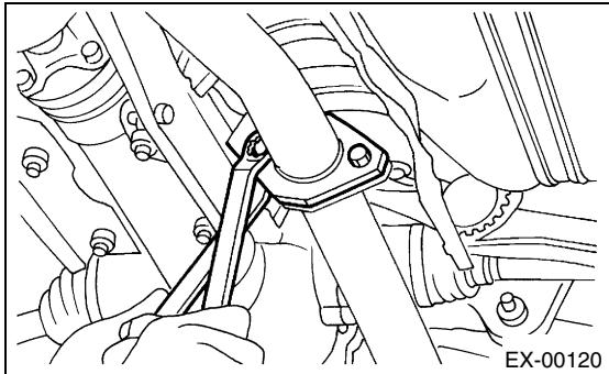
2) Remove the rubber cushions, and detach muffler.
