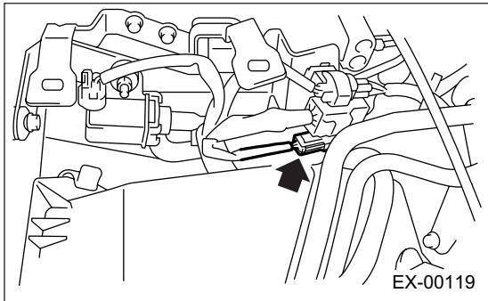
4) Remove the front oxygen (A/F) sensor. <Ref. to FU(H4DOTC)-45, REMOVAL, Front Oxygen (A/F) Sensor.>
