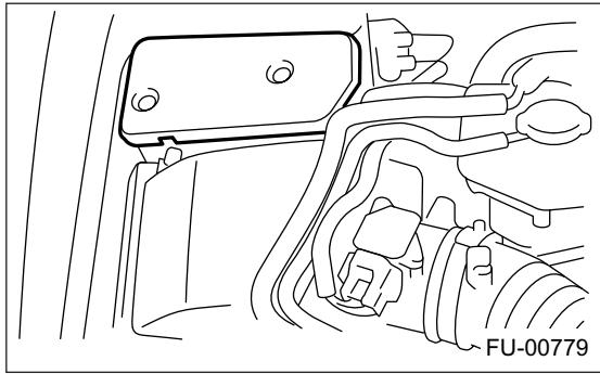
3) Disconnect the exhaust temperature sensor connector.
