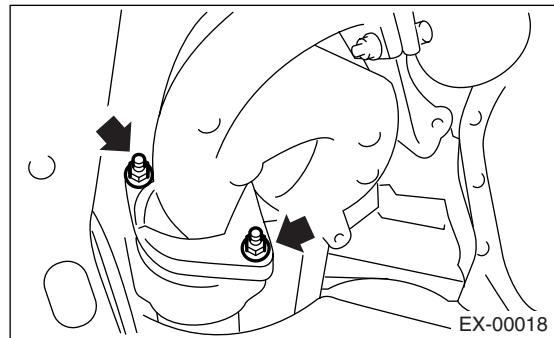
8) Remove the center exhaust pipe. <Ref. to EX(H4DOTC)-8, REMOVAL, Center Exhaust Pipe.>
