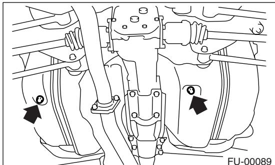
6) Tighten the fuel drain plug.
