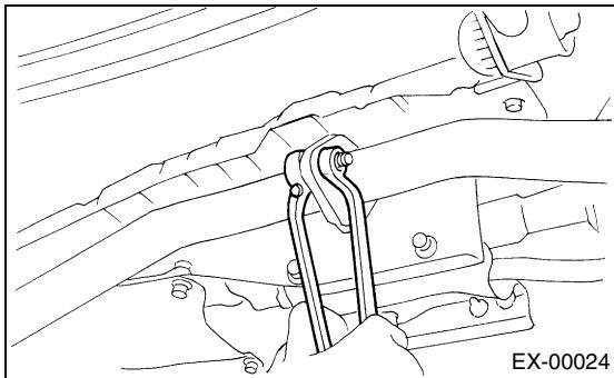
2) Apply a coat of SUBARU CRC to mating area of the cushion rubbers in advance.
