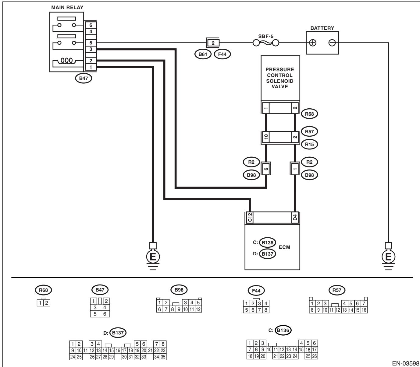
**DIAGNOSTIC PROCEDURE WITH DIAGNOSTIC TROUBLE CODE (DTC)**
