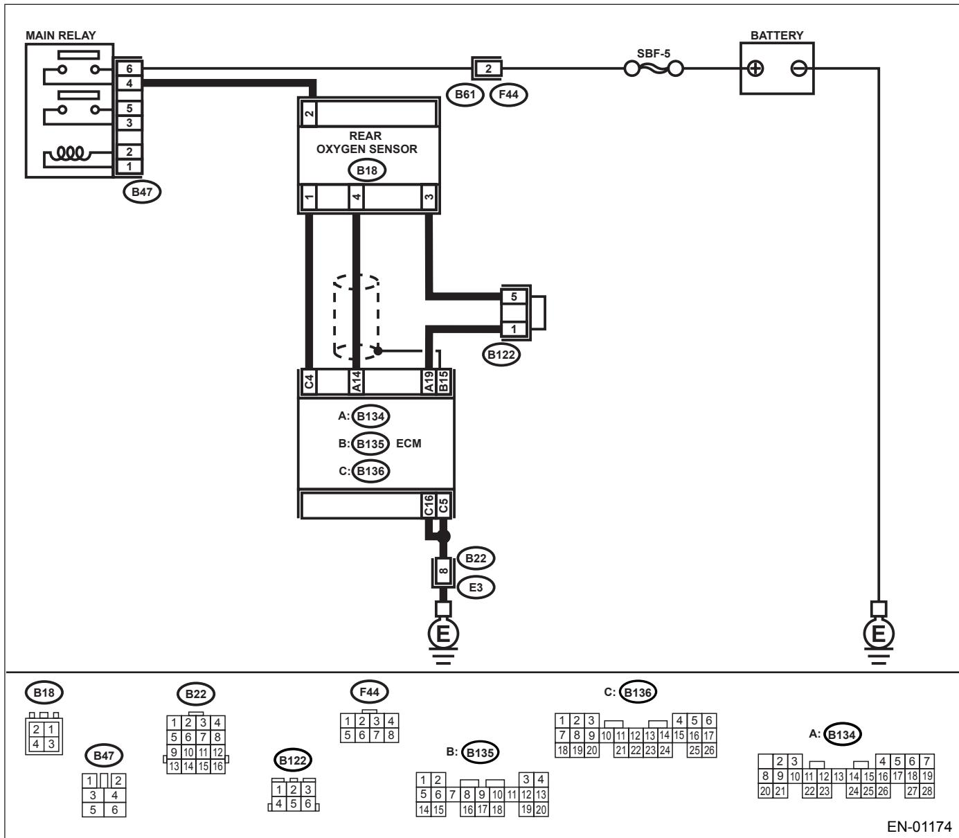
**DIAGNOSTIC PROCEDURE WITH DIAGNOSTIC TROUBLE CODE (DTC)**
