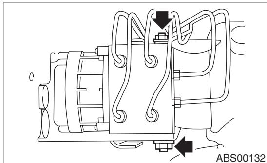
3) Connect the brake pipes to their correct ABSCM&H/U connections.
