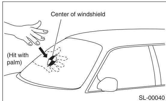
If NG, adjust the impact sensitivity. <Ref. to SL-49, ADJUSTMENT, Security Control Module.>
