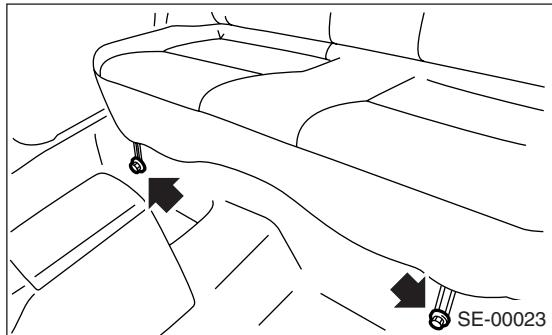
2) Remove the bolts securing lower portion of backrest and then open the center trunk through lid.
