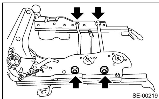
8) Loosen two bolts to remove the slide rail.
