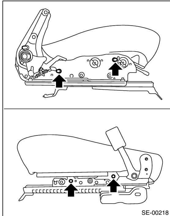
7) Loosen four screws to remove the hinge.
