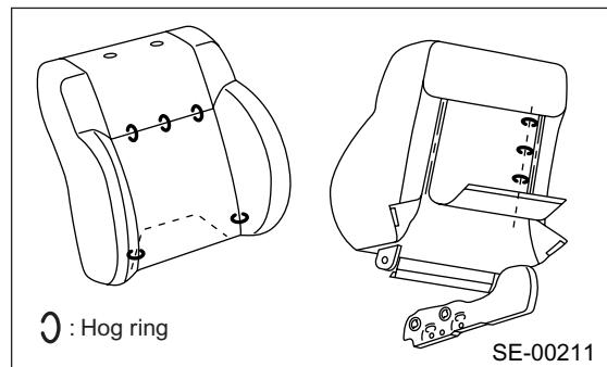
10) Remove the hog rings, and then remove the seat cushion cover.
