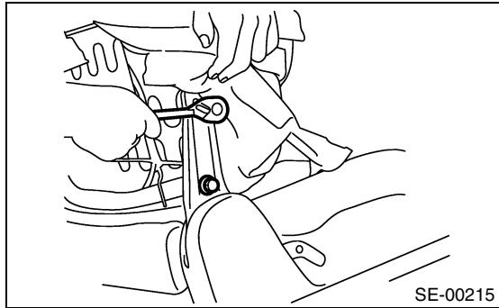
4) Remove the hinge screw cover and screw, and remove seat back rest from hinge.
