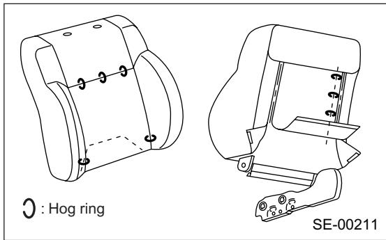
9) Remove the hog rings, and then remove the seat cushion cover.
