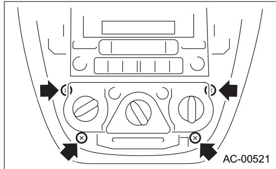
7) Pull out the control unit and disconnect connectors.
