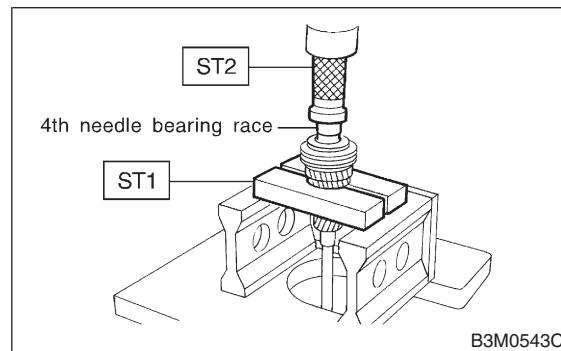
4) Install baulk ring, needle bearing (32 × 30 × 25.7), 4th drive gear and 4th gear thrust washer to transmission main shaft.
