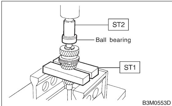
6) Using ST1 and ST2, install the 5th gear thrust washer and 5th needle bearing race onto the rear section of transmission main shaft.
