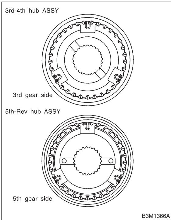
2) Install 3rd drive gear, outer baulk ring, synchro cone, inner baulk ring, sleeve and hub assembly for 3rd needle bearing on transmission main shaft.
