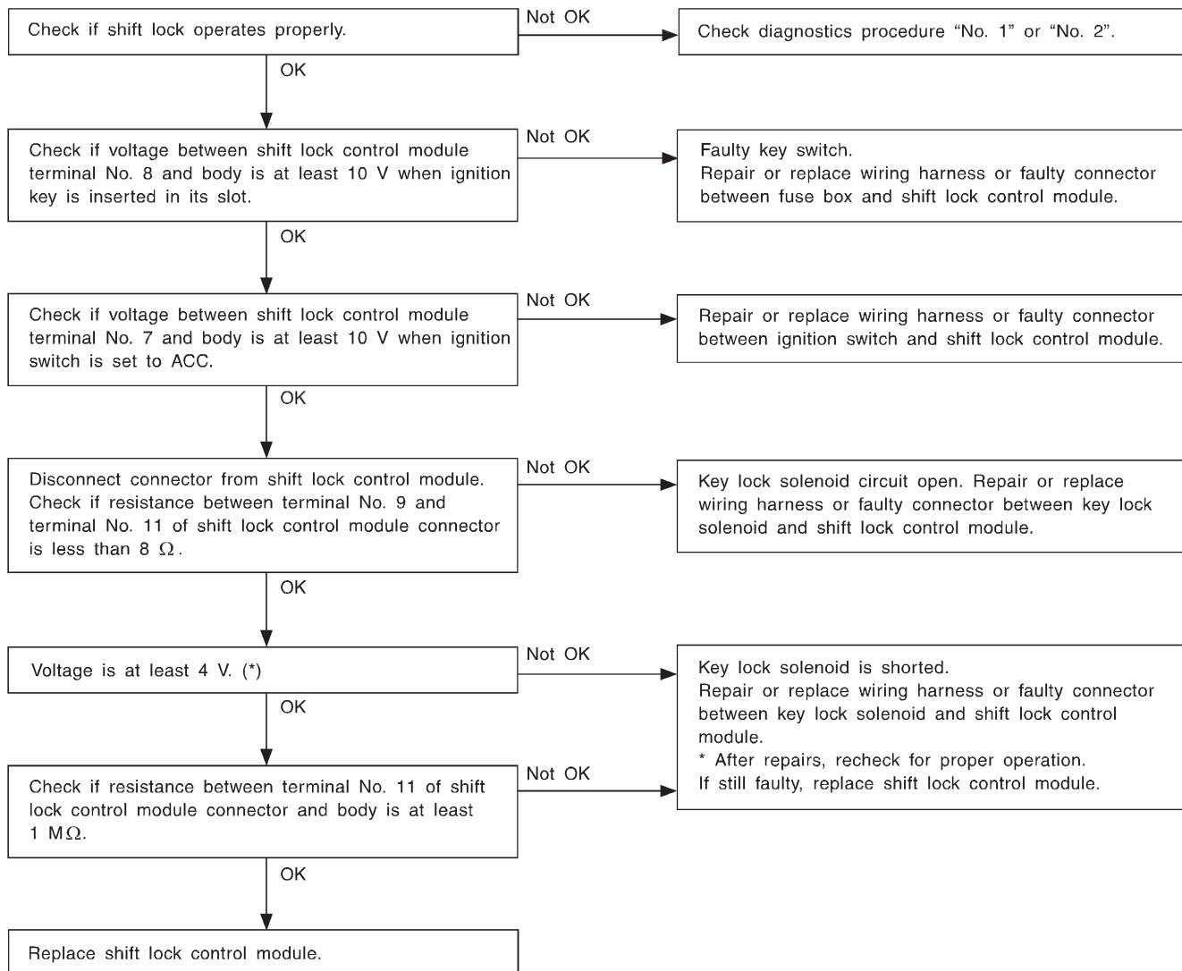
\*: When conducting operational checks of the key lock solenoid, do not apply 12 V to solenoid for more than one second, since this may break solenoid circuit.
