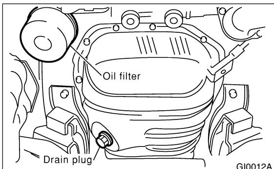
5) Fill engine oil through filler pipe up to upper point on level gauge. Make sure that vehicle is placed level when checking oil level. Use engine oil of proper quality and viscosity, selected in accordance with the table in figure.
