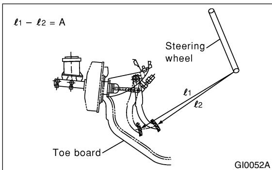
4) Check to see if air is in the hydraulic brake line by the feel of pedal operation. If air appears to exist in the line, bleed it from the system.
