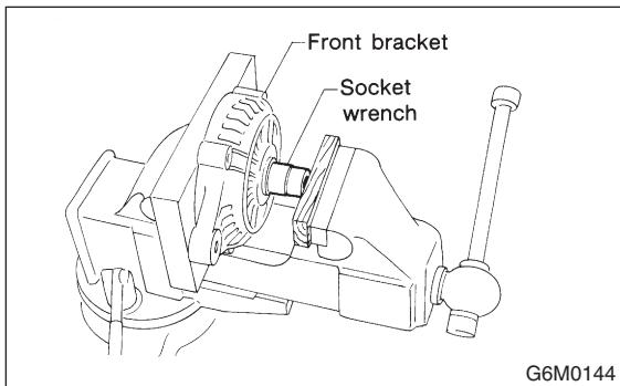
(3) Set a new bearing and closely install a fit tool on the bearing outer race. Press the bearing down into place with a hand press or vise. A socket wrench can serve as the tool.
