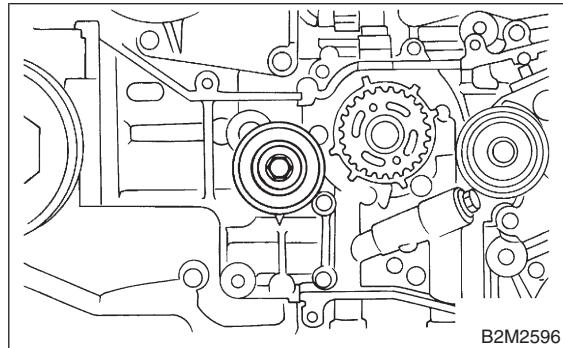
2) Remove automatic belt tension adjuster assembly.
