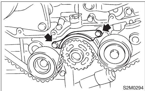
2) If alignment mark (a) and/or arrow mark (which indicates rotation direction) on timing belt fade away, put new marks before removing timing belt as shown in procedures below.
