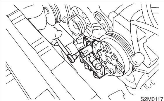
16) Remove oil pump by using flat bladed screwdriver.
