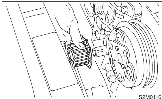
15) Remove bolts which install oil pump onto cylinder block.
