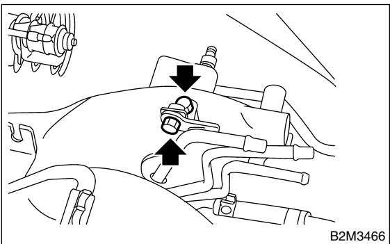
18) Remove bolt which installs injector pipe on intake manifold.
