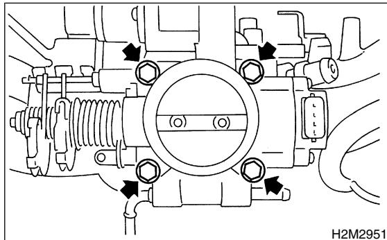
23) Connect connector to throttle position sensor and idle air control solenoid valve.
