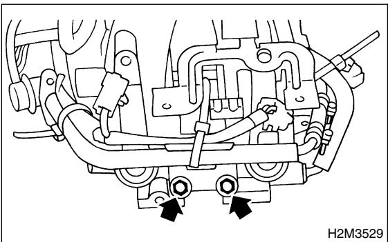
19) Remove fuel injector while lifting up fuel injector pipe.
