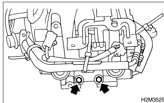
9) Tighten bolt which installs injectors pipe on intake manifold.
