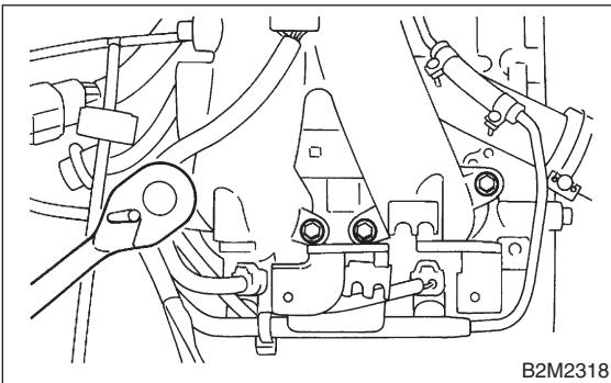
20) Remove intake manifold.
