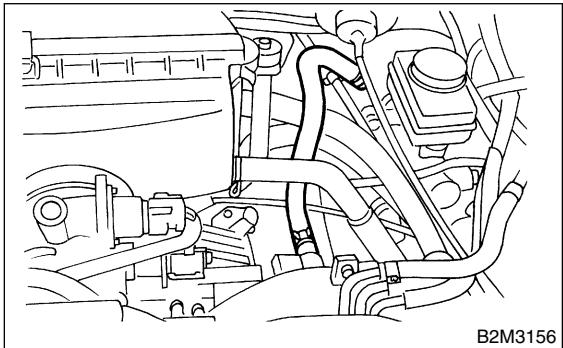
10) Connect engine coolant hose to throttle body.
