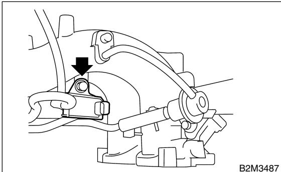
20) Remove bolt which installs injector pipe on intake manifold as shown in figure.
