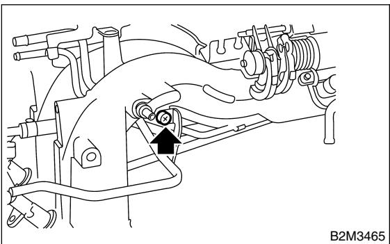
17) Remove two bolts which hold fuel pipes on the left side of intake manifold.
