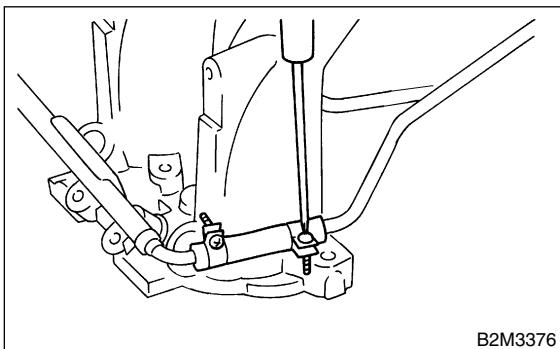
4) Install fuel injector pipe.
