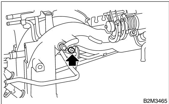
12) Install purge control solenoid valve.
