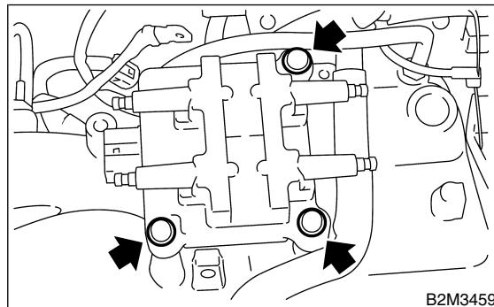
24) Connect connector to ignition coil and ignitor assembly.
