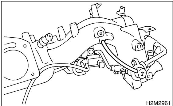
19) Install air assist injector solenoid valve to bracket.
