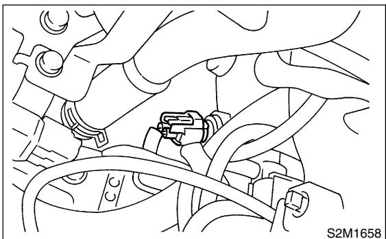
8) Install air cleaner case stay RH and engine harness bracket, and connect engine harness connectors to bulkhead connectors.
