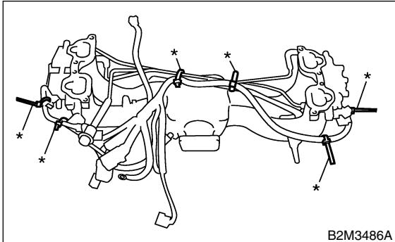
18) Remove engine harness from intake manifold.
