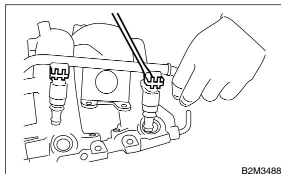
8) Tighten bolt which installs injector pipe on intake manifold.
