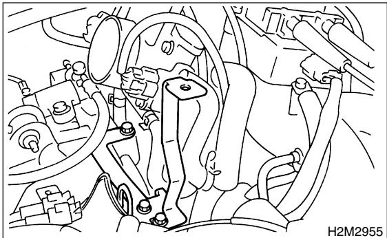
13) Disconnect connectors from engine coolant temperature sensor.
