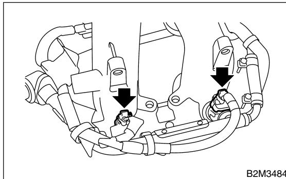
15) Disconnect connector from purge control solenoid valve.
