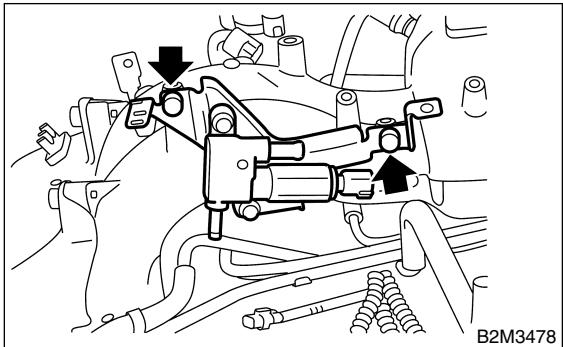
20) Connect air by-pass hoses to air assist solenoid valve.
