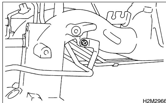
22) Remove two bolts which hold fuel pipes on the left side of intake manifold.
