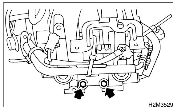
9) Tighten bolt which install injector pipe on intake manifold.
