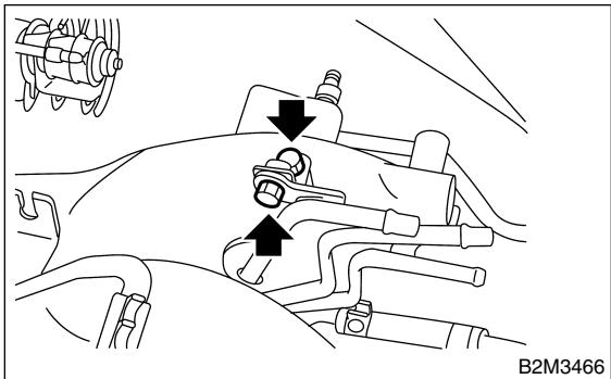
11) Tighten bolt which install injector pipe on intake manifold.
