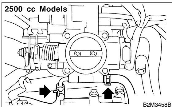
11) Connect PCV hose to intake manifold.
