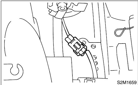
15) Disconnect connector from crankshaft position sensor.
