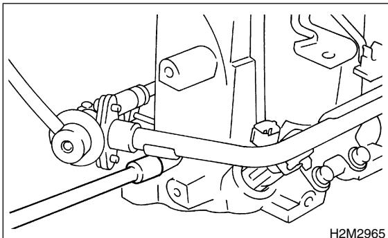
21) Remove bolt which installs injector pipe on intake manifold.
