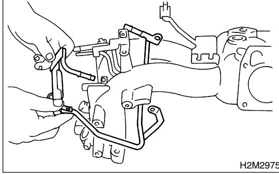
24) Remove bolt which installs fuel pipes on intake manifold.
