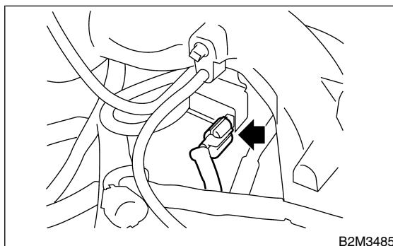
16) Disconnect air by-pass hose from purge control solenoid valve.
