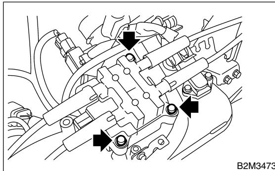
28) Connect connector to ignition coil and ignitor assembly.
