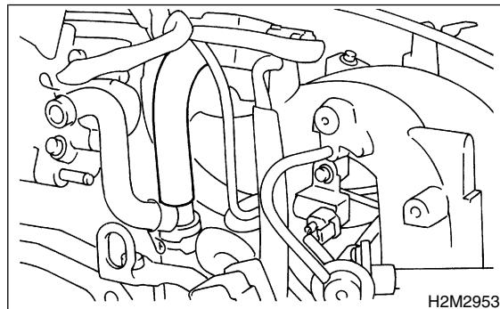
10) Disconnect engine coolant hose from throttle body.
