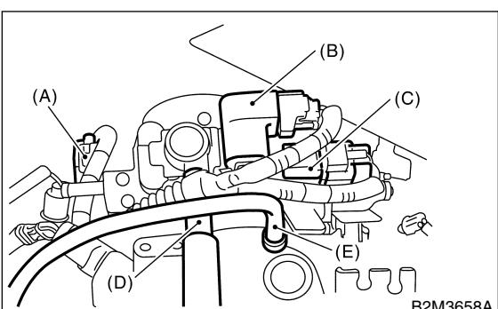
23) Install ignition coil and ignitor assembly.
