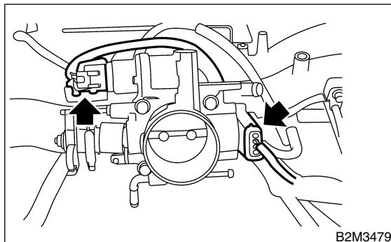
24) Connect air by-pass hose to throttle body.
