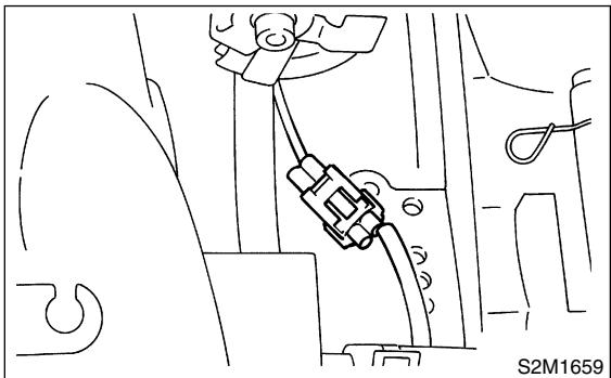
7) Connect connectors to engine coolant temperature sensor.
