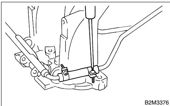
4) Install fuel injector pipe.
