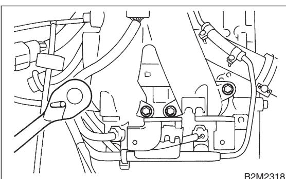
5) Connect connector to crankshaft position sensor.
