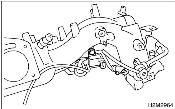
13) Connect hoses to purge control solenoid valve.
