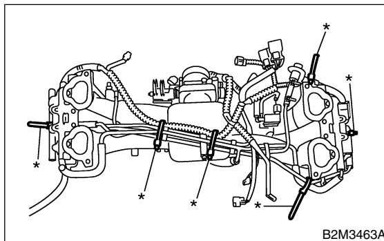
13) Remove engine harness from intake manifold.
