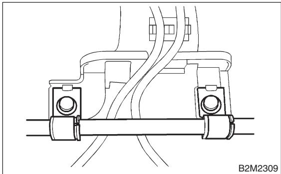
(5) Remove bolts which install power steering pump to bracket.
