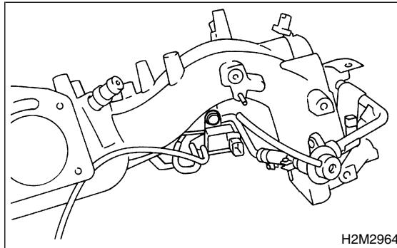
15) Remove bolt which installs injector pipe on intake manifold as shown in figure.
