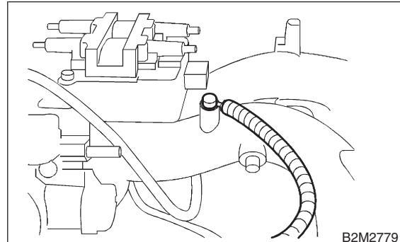
2) Disconnect connector from ignition coil and ignitor assembly.
