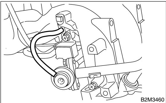
19) Install throttle body to intake manifold.
