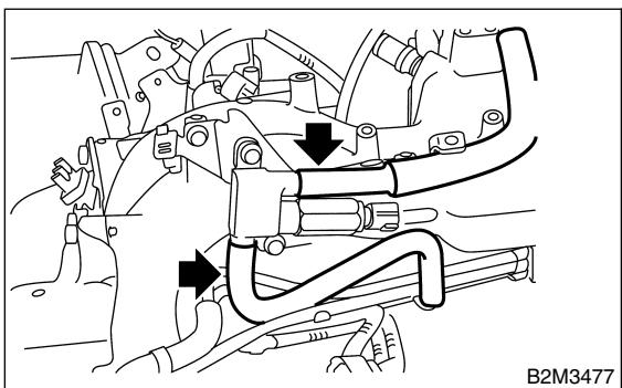
11) Remove air assist injector solenoid valve from intake manifold.
