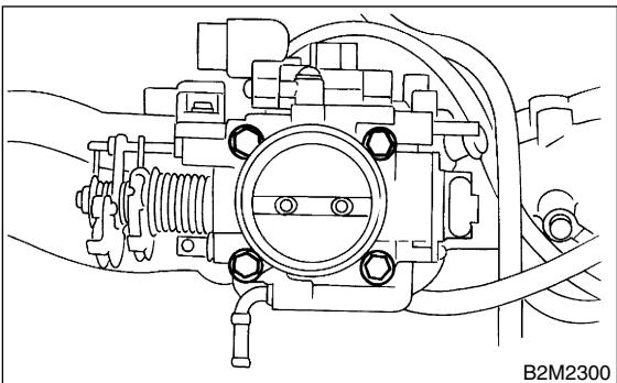
20) Connect connectors to throttle position sensor (A), idle air control solenoid valve (B) and intake manifold pressure sensor (C).
