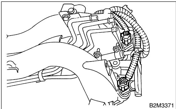
11) Disconnect connector from purge control solenoid valve.
