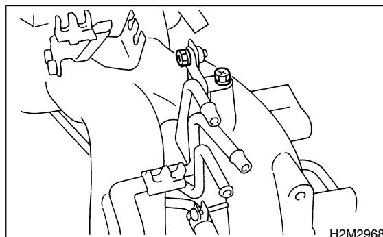
23) Remove bolt which installs injector pipe on intake manifold.
