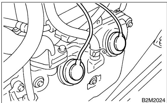
9) Disconnect PCV hose from intake manifold.
