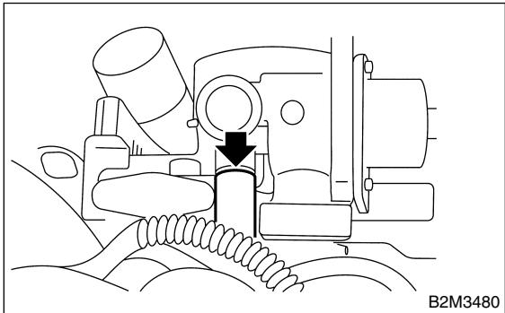
25) Install intake air temperature and pressure sensor.
