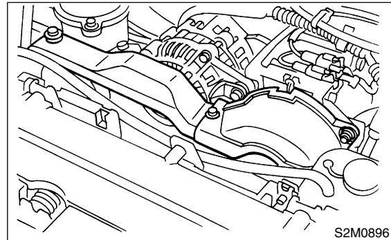
(6) Install resonator chamber.
