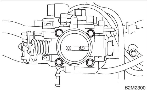
8) Disconnect pressure regulator vacuum hose from intake manifold.
