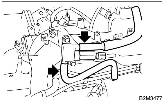
21) Connect connector to air assist solenoid valve.
