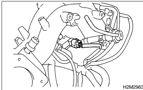
12) Remove harness bands (\*) which hold engine harness onto intake manifold.
