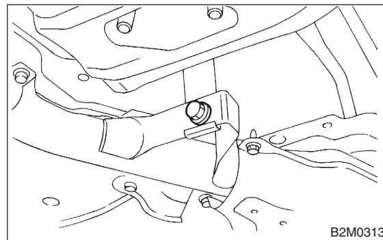
4) Tighten bolts which hold front exhaust pipe onto cylinder heads.
