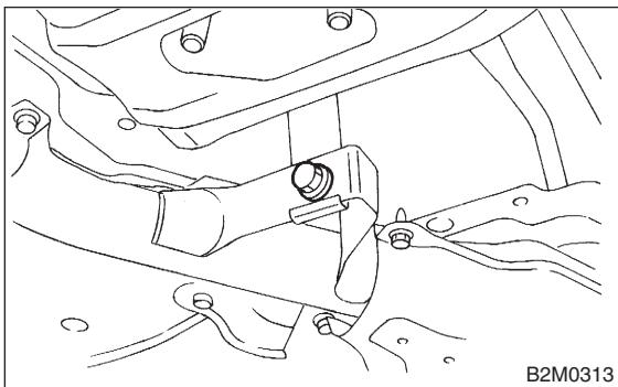
7) Connect rear oxygen sensor connector.
