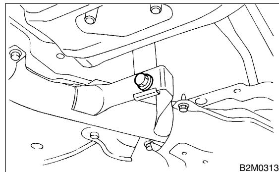
8) Remove front and center exhaust pipe assembly from the vehicle.
