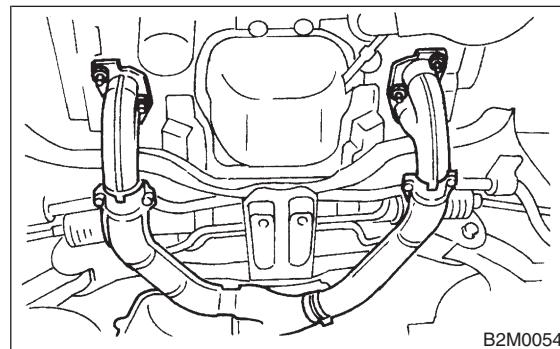
5) Tighten bolts which install front and center exhaust pipe assembly to rear exhaust pipe.
