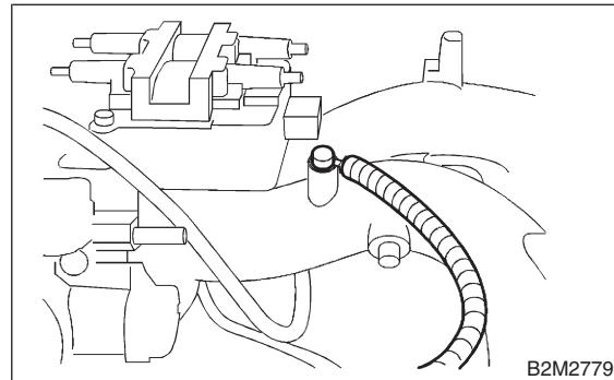
10) Use TCM mounting stud bolts at the body head grounding point when measuring voltage and resistance inside the passenger compartment.
