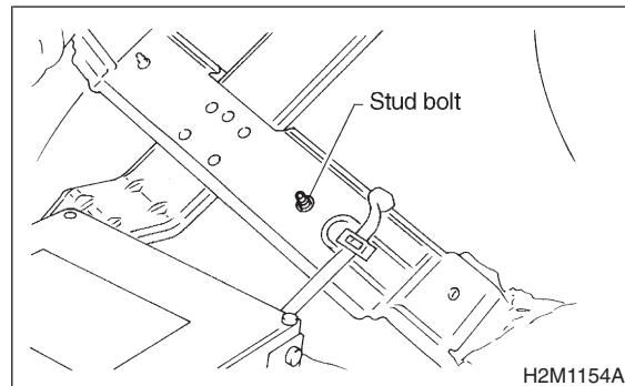
9) Use engine grounding terminal or engine proper as the grounding point to the body when measuring voltage and resistance in the engine compartment.
